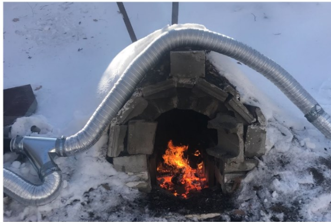
Forge in operation during initial ventilation tests
