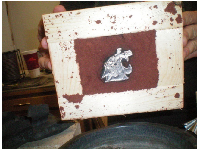
Figure 2. Aluminum screaming cougar head cast from aluminum into a sand mold during MSE day.
